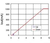
Dimming curve with analog PWM
