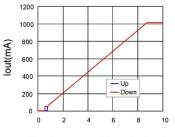
Dimming curve with analog input
