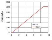
Dimming curve with analog input
