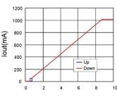
Dimming curve with analog PWM
