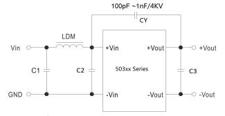
C1,C2: 4.7uF/25V CY: 100pF ~ 1nF/4kv LDM: 6.8uH C3: 1uF to 10uF/16V
